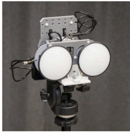
Figure 3: Photograph of long-range FMCW radar, SNR vs. distance for different RCS, and some key parameters of the radar system.
