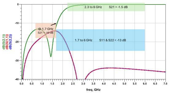
Figure 2. Design rules of S21 and S11 in the stopband and passband
