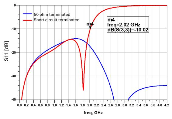
Figure 4. Evaluation example for short circuit termination (Simulated data: Blue curve is 50  $\Omega$  terminated, red curve is short terminated.).
